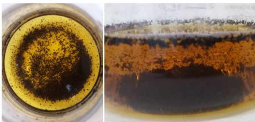
Figure 4: Reaction system after catalytic decomposition experiment of H_2O_2 by iodide ions in the presence of methylene blue
